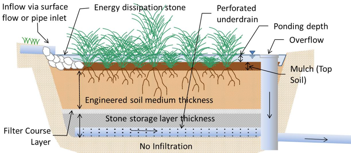
FIGURE 5-9. Schematic of a Typical Biofiltration Basin
