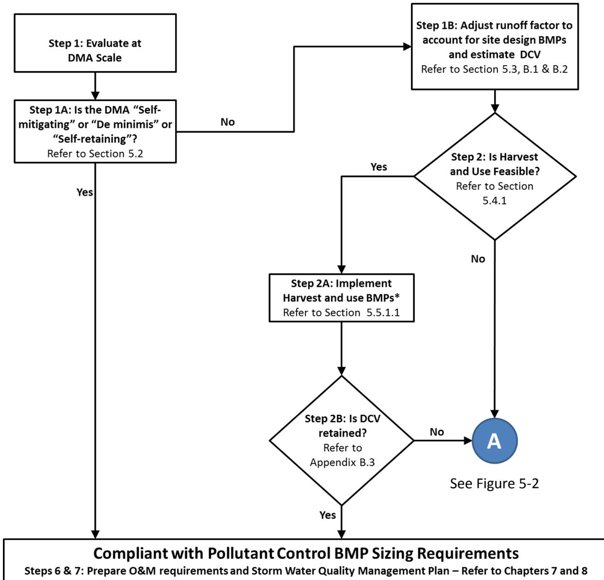
\* Step 2C: Project applicant has an option to also conduct feasibility analysis for infiltration and if infiltration is fully or partially feasible has an option to choose between infiltration and harvest and use BMPs. But if infiltration is not feasible and harvest and use is feasible, project applicant must implement harvest and use BMPs
