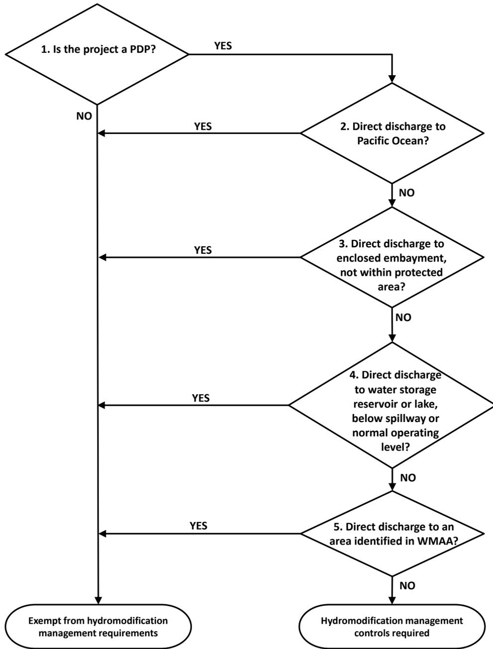
\*Direct discharge refers to an uninterrupted hardened conveyance system; Note to be used in conjunction with Node Descriptions.
