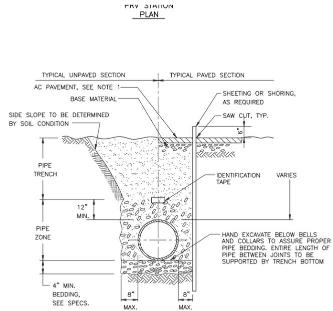
TYPICAL TRENCH SECTION DETAIL 2 C-2
